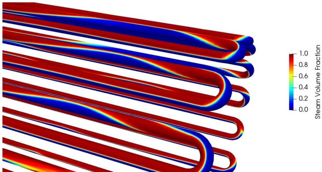
*Figure 23: Vapor phase fraction contour within radiant tubes*
