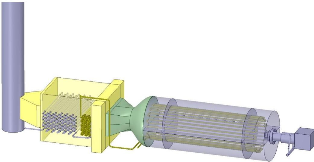
*Figure 3: OTSG CAD Model including Fire Side and Water Side*
