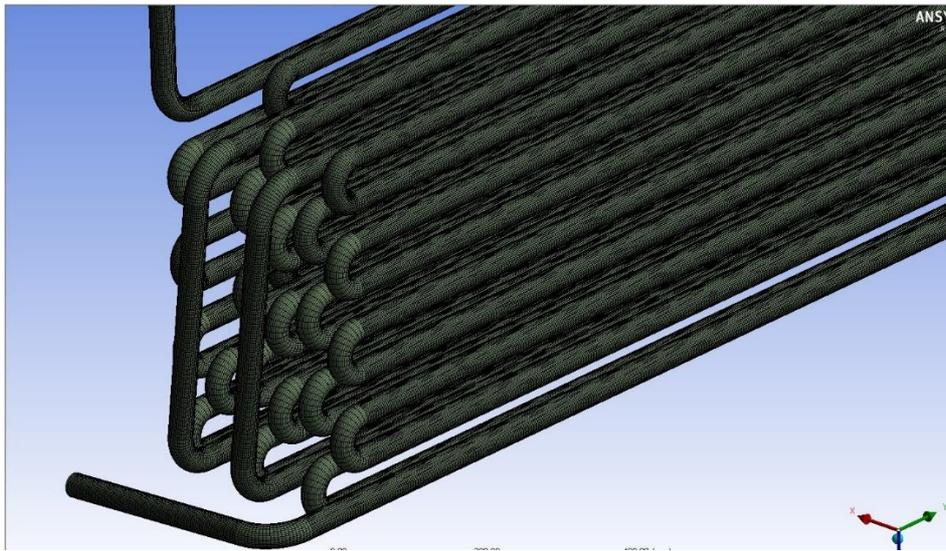
*Figure 13: Mesh Grid for Second Convection Tubes (First Tubes)*
