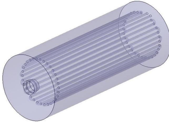
*Figure 6: Radiant Section of OTSG – solid model [Transparent mode is shown to visualize the steam tubes inside the furnace]*
