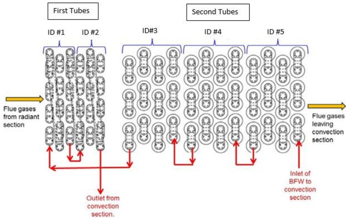
Figure 2: Tubes and flow arrangement in convection section
