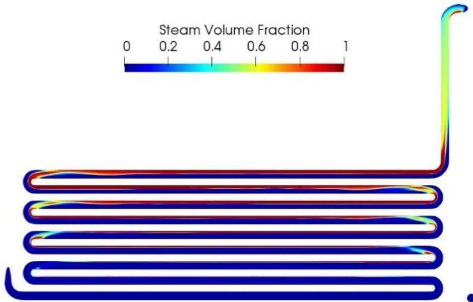
Figure 22: Vapor phase fraction contour within second convention tubes in convention box on a vertical cut
