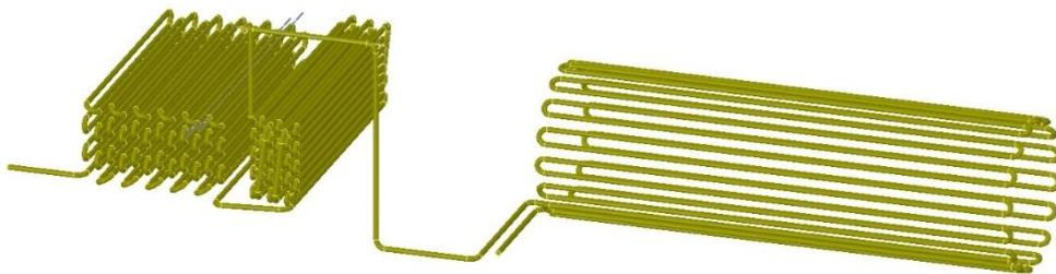
*Figure 8: Tubes CAD model for Water Side*
